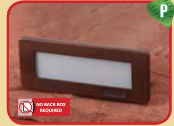
SL-08AL-LEDP-BAR: NO BACK BOX REQUIRED 12v Driver Supplied Cast aluminum or brass 12v 8w integrated flat panel LED 50,000 hours average rating 3000K warm white or 5200K cool white External 12v AC driver required (supplied)
