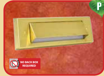
SL-04-1L-LEDP-BRS: NO BACK BOX REQUIRED 12v Driver Supplied Aluminum, brass, copper or stainless steel 12v 8w integrated flat panel LED 50,000 hours average rating 3000K warm white or 5200K cool white External 12v AC driver required (supplied)
