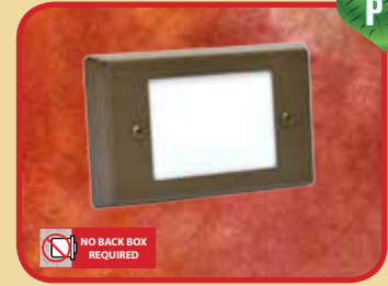
SL-02-AL-LEDP-WBR: NO BACK BOX REQUIRED 12v Driver Supplied Aluminum, brass, copper or stainless steel 12v 4w integrated flat panel LED 50,000 hours average rating 3000K warm white or 5200K cool white External 12v AC driver required (supplied)
